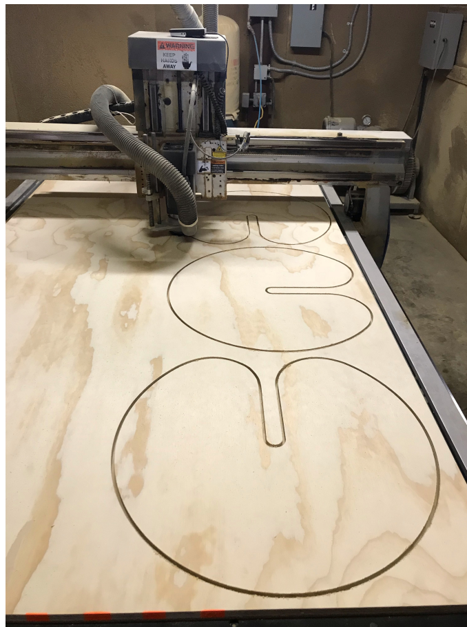
Figure 2 LilPads Being Cut Out on CNC
