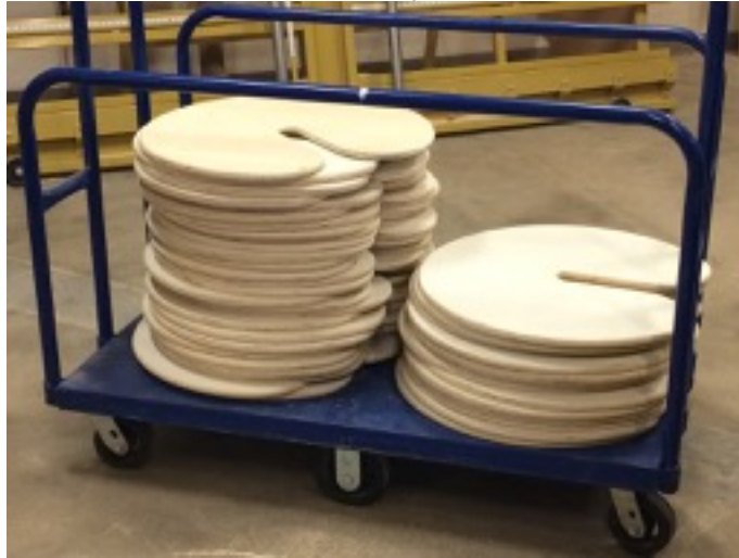
Figure 3 Completed LilyPad Blanks (After CNC and Edge Rounding)
